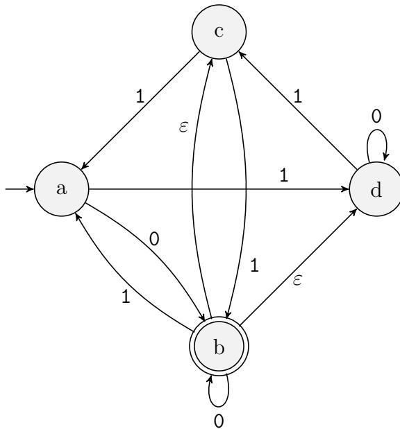
(b) Use the table from part b to convert  $N$  to an equivalent DFA  $M$  using the method of subset states. Draw  $M$ 's state diagram.
